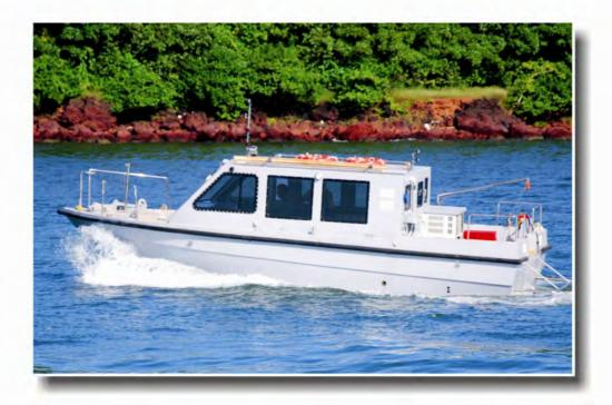
The boat is capable of carrying out Hydrographic survey operations using modern surveying equipment / system, up to a minimum water depth of one meter below hull mounted single beam echo-sounder transducers. It shall also be able to undertake emergency operations like landing shore survey parties and providing logistic support to shore camps.
