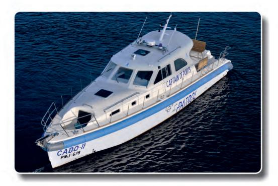
The boat is a day / night surveillance and investigation vessel operating in shallow coastal waters in and around harbour and anchorage. The boat is highly seaworthy, unsinkable type and is able to sustain operations up to sea state 3 in open sea and also in breaking sea waves near the coast while in shallow water. The boat has propulsion & power generation, life saving & ballistic protection and other engineering and electrical systems to carry out safe and reliable operations.
