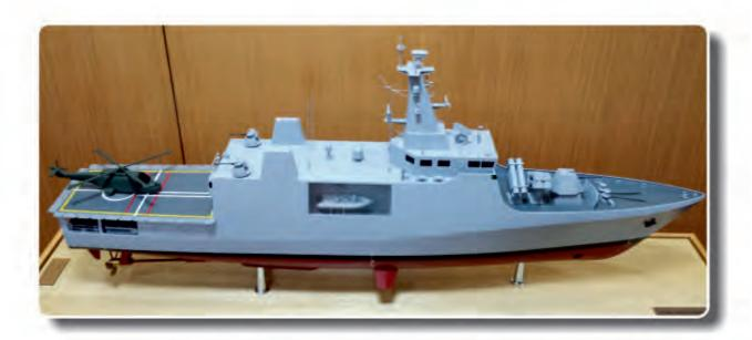
This mid-sized Offshore Patrol Vessel, 75m in length, is a new in-house designed product of Goa Shipyard Limited, capable of undertaking day and night patrolling and policing operations, search and rescue operations, embarkation & operation of upto 5.5 Ton helicopter for long range all time search & rescue and surveillance.
