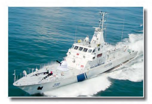
This 35 Knots, 50 meters in length, Fast Patrol Vessel, is in-house designed and built by Goa Shipyard Ltd. This vessel is primarily designed for patrolling, anti-smuggling and anti-terrorist operations. It can also support the Navy during wartime as a coastal convoy escort and as a communication link.
