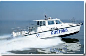
The Fast Interceptor Boat (FIB) is capable of performing high speed pursuits and interception in various border protection roles including anti-smuggling, anti-infiltration, fisheries, patrol and immigration and anti-terrorism activities. The vessel can also be used for search and rescue operations.
