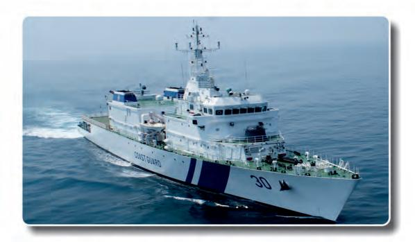
This Offshore Patrol Vessel, 90m in length, is an in-house designed product of GSL, capable of patrolling and policing operations, search and rescue operations, embarkation & operation of ALH helicopter for long range all time search, rescue & surveillance, pollution response against oil spillage and external fire-fighting.
