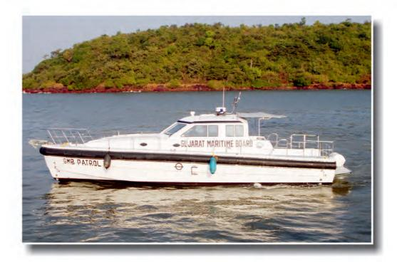
The Patrol Boat is a hard chine mono hull form that has been proven under offshore conditions and gives an outstandingly seaworthy boat with predictable and excellent handling agility at all speeds.
